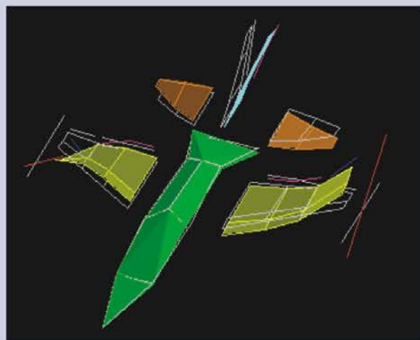
Deformation mode shape of an F16 wing
