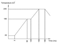
Wave soldering: Temp. peak up to 260 ℃ allowed for 5s (on pins)
