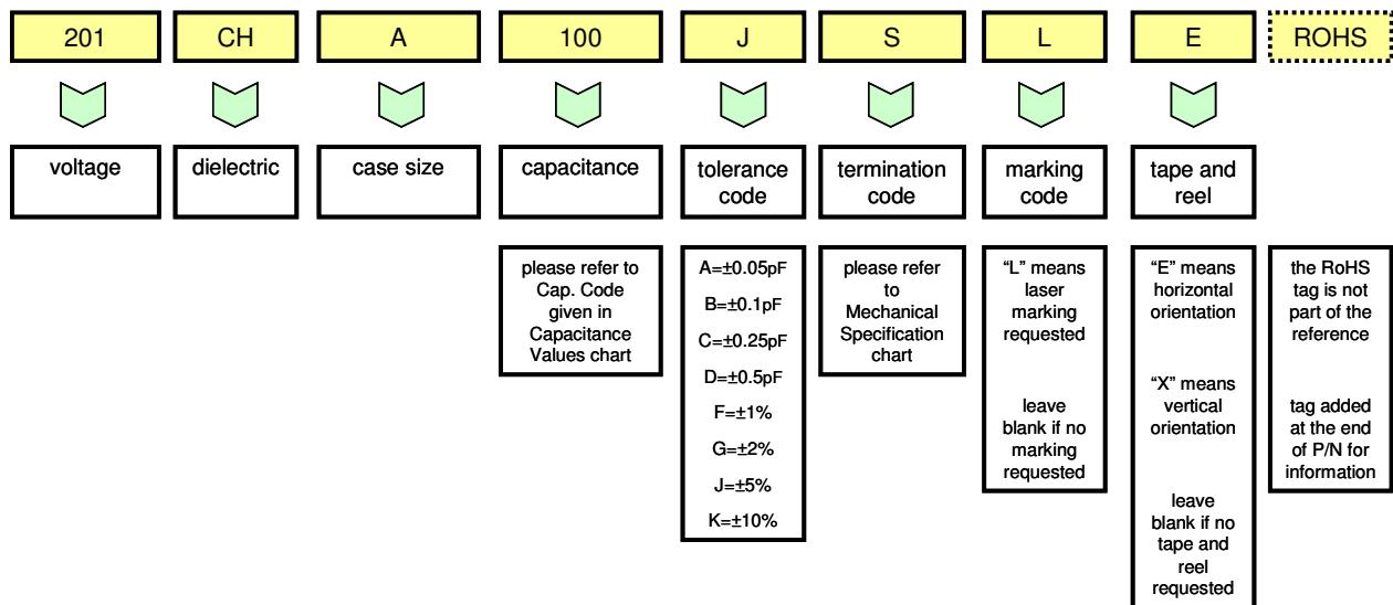
NB: for capacitance values lower than 10pF, tolerances A, B, C and D apply. For capacitance values equal to or higher than 10pF, tolerances F, G, J and K apply;
